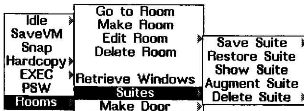
Figure 7-1. The ROOMS "Suite" command and the suite submenu. Selecting "Suites" opens the suite submenu.
