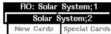
Figure 12-8. The notefile Banner after compacting to the same file name. The old version is "Solar System;1." The new version is "Solar System;2."
