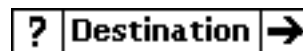
Figure 8-28. A cross-file link to a closed notefile. The question-mark bitmap indicates that the card cannot be accessed to determine its card type.
