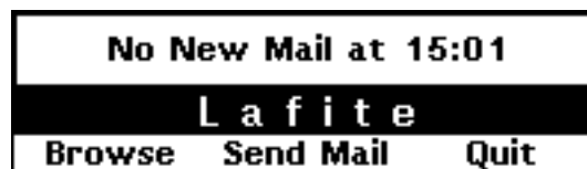
Figure 2. The status window, showing the status region, the title bar, and the menu of commands
