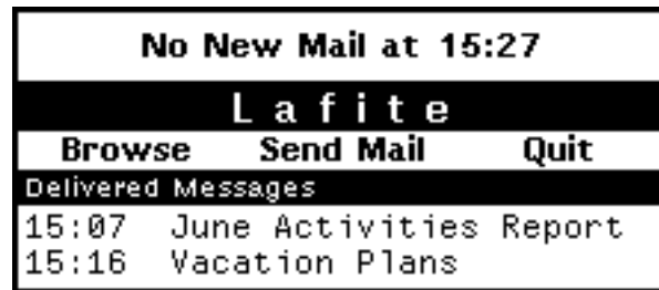
Figure 25. A status window showing the out-box. The number of messages retained can be changed using the LAFITEOUTBOXSIZE variable; see chapter 13, "Customizing Lafite"
