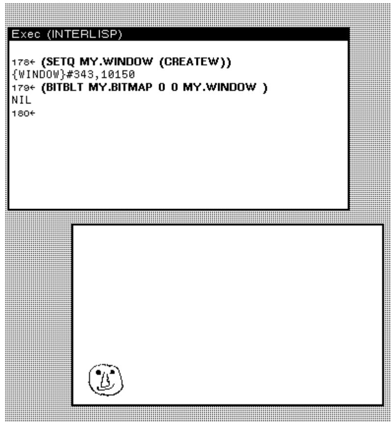
Figure 14-5. BITBLTing a Bitmap onto a Window
